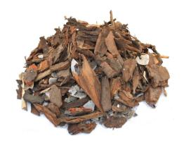
BioFilm is Azwood's biofilter media for effective control of volatile organic compounds (VOCs). A biofilter is a natural and sustainable solution designed to tackle odours from wastewater treatment facilities, compost facilities, rendering plants, and other odour-producing operations.
